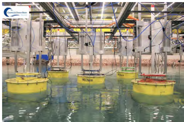
The experimental setup of the five-WEC array the Coastal and Ocean Basin Ostend: overview (left) and detail (right).
