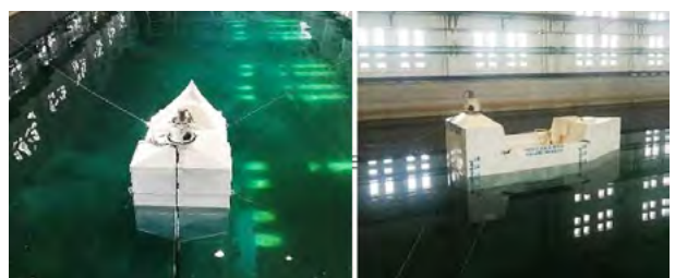
GIEC Single floating OWC device test
