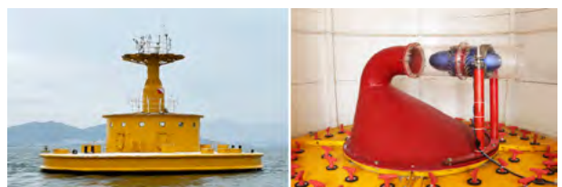
OWC ocean buoy in sea trial operation
