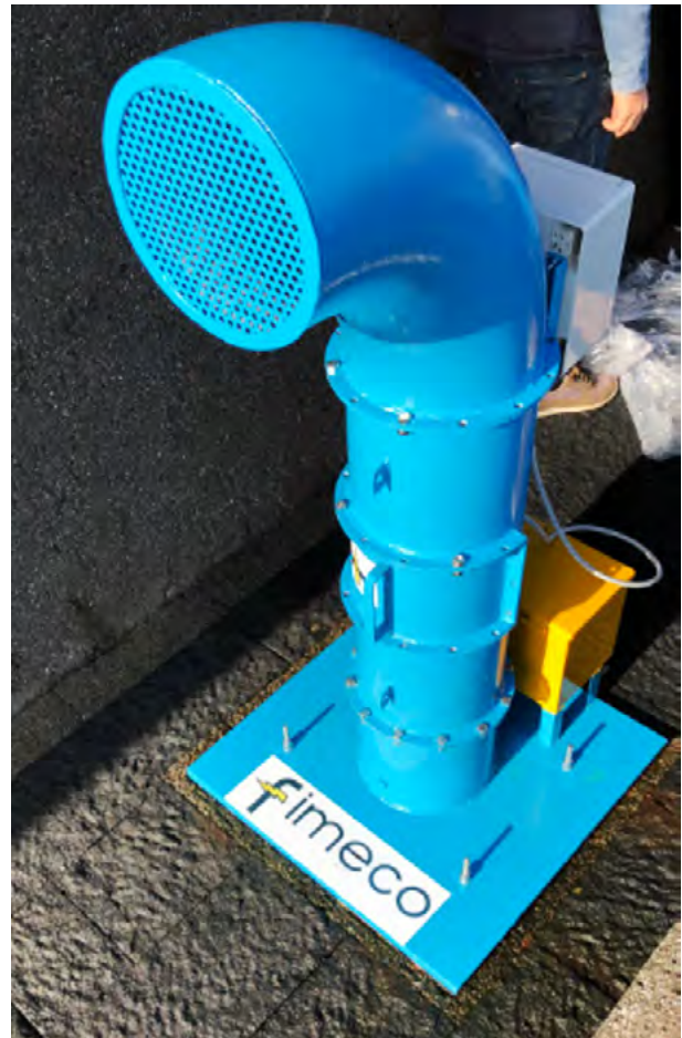
The turbine developed by Fimeco and Enermedesea installed in Lipari island breakwater barrier
