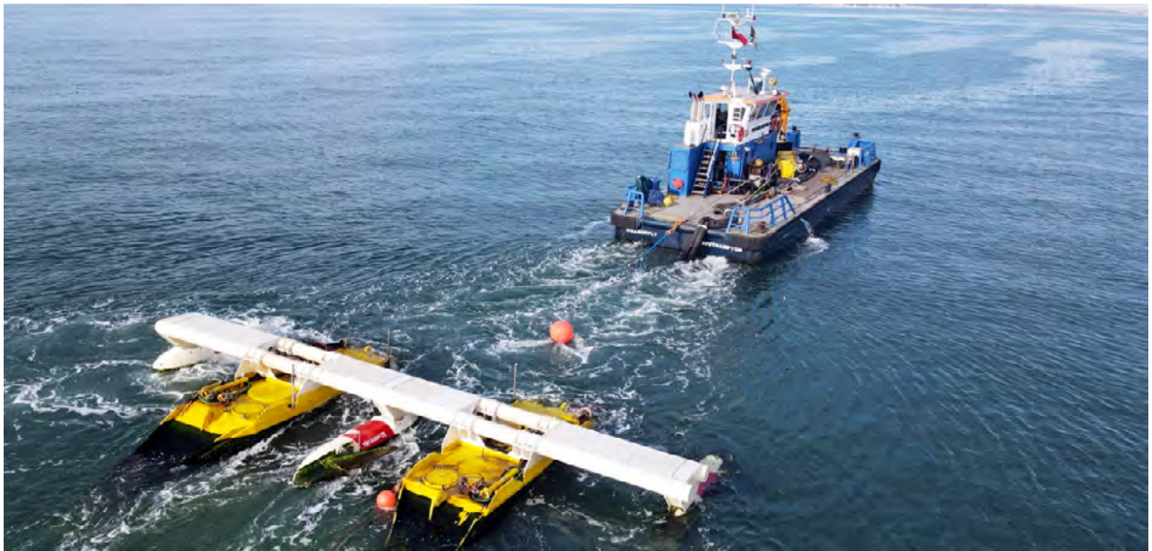
QED Naval Subhub being towed to Langstone as part of TIGER Project. Photo: © QED Naval.
